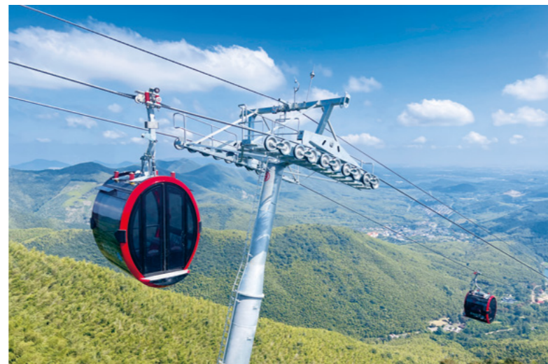
Detachable 8-Seater Gondola Lift | Yixing Bamboo Sea Park | China Design by Studio F. A. Porsche
